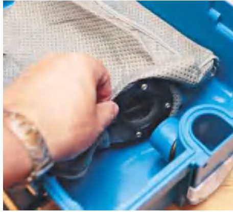
▲ The neoprene bag slips over the air inlet spigot and is reusable
